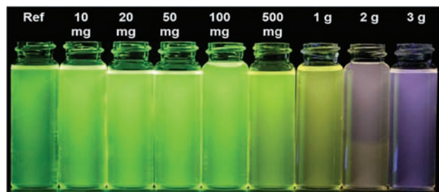
Figure 1. Photograph of solutions containing XF1 and increasing concentrations of phenylacetic acid. Photographs were taken under a hand-held blacklight at a wavelength of 366 nm.
